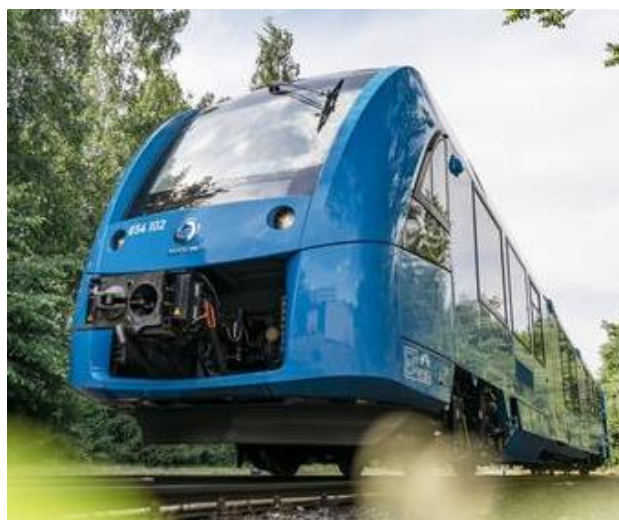
Figure 26 – Alstom Hydrail with Hydrogenics Engine (Photo courtesy of Alstom) 2
